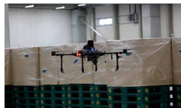
A drone operating semi-autonomously, using a laser sensor to determine the positional relationship between cargo and the floor on a test course using pallets to simulate cargo
