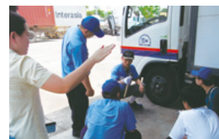
Inspecting tires, wheels, etc., using inspection hammer
