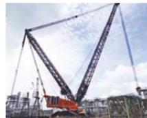
Crawler crane able to hoist 1,350 tons
