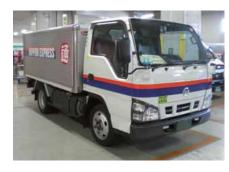
Engines are fuelled with liquefied petroleum gas, which is commonly used by taxis. Compared to diesel engines, NOx emissions are far lower and there is no PM exhaust. Because more and more fuelling stations (LPG stations) are found nationwide, we have increased the number of LPG trucks in the fleet.
