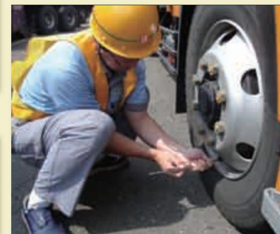
Air pressure measurement (pen-type gauge)
