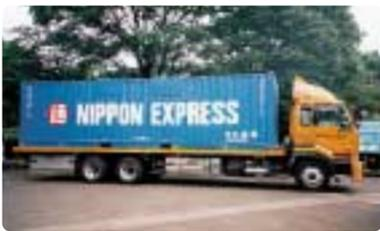
The first large truck in Japan to be powered by CNG (compressed natural gas)
