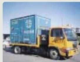
CNG-powered large truck (JR 5-ton single container model)
