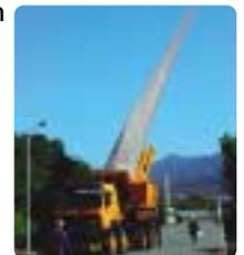
Wind turbine blade transport using our blade vertical transport system.
