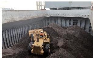
Onboard wood fuel trimming operations
